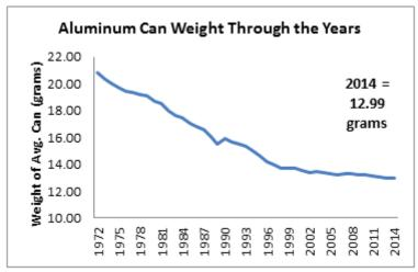
the weight, while improving the mechanical properties so that the thinner material making the can still carries out all of the requirements of a can.
