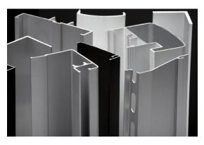
Less fabrication and machining after extrusion means that there is greater design potential because intricate shapes may be extruded, reducing the need to manufacture component parts for future assembly. Some shapes achievable by extrusion are unattainable by any other process.
