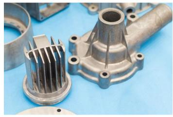
Special techniques, such as vacuum diecasting may reduce these entrapped gases. Aluminium alloy
