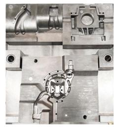
pressure during the solidification process. The extent of pressure applied is significantly less than that in forging. Fine highly detailed parts can be produced, and coring can be used in tandem with the process to form holes and recesses.
