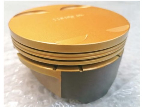
• Diamondyzed + coated piston after coating top with ceramic gold coat and skirt with lube
