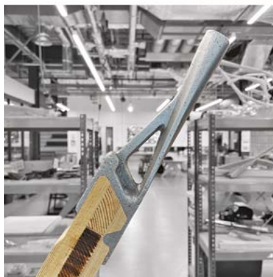
• Right: Cast and machined component for shelter project by students on the design for manufacture course (2021)
