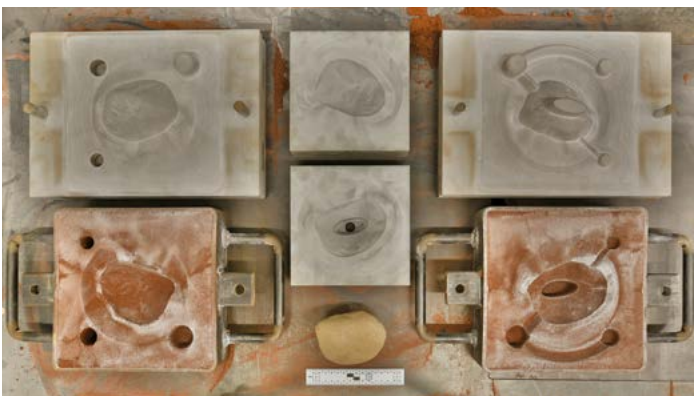
• Above: Set of patterns for cope, drag core box to sand mould the “Pebble” project by Melis Van Den Berg (2021)”
