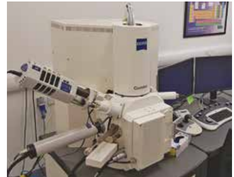
Figure 1: (Above & opposite); One of our advanced characterisation equipment for studying microstructure is our FEG-SEM Zeiss with EBSD and EDS.
