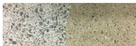
Pictured above, a section through a test panel of PBond Solo 60GM on a mullite based low cement castable. The sample was cut after firing to show adhesion to fracture surface of existing castable.
