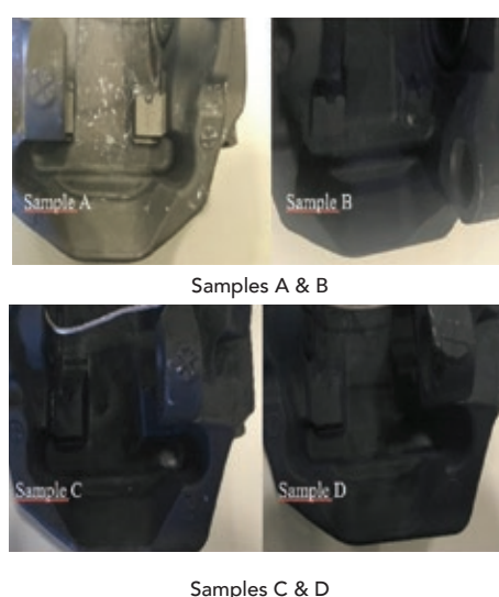
Figure 5 NSS results of Sample A, B, C and D after subjecting to NSS for 800 hours according to ISO 9227
