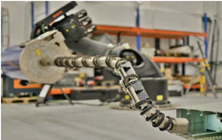
Figure 3: Purpose-built OC Robotics snake robot inspecting the mid-section of an A320 Airbus wing. 3DIMPact Research Group (Prof Stuart Robson)
