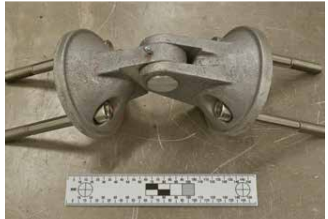
Figure 4: Cast aluminium nodes for a timber structure designed and modelled by Christopher Leung of the Bartlett and sand cast by Melis Van Den Berg of B-MADE at HereEast, UCL, London
